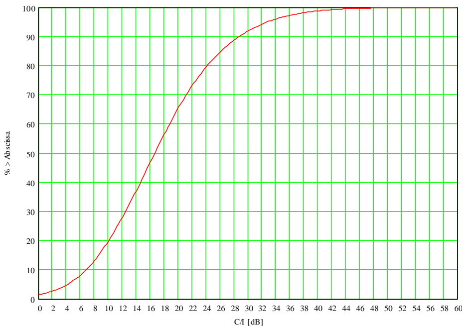
Figure X.19 C/I CDF for an N=7 omni network with an interfering Normal BTS that is radiating intermodulation emissions at 50 dB rms below the Microcell EIRP, standard deviation = 6 dB.
