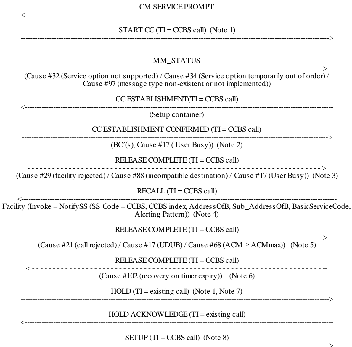
Figure 4.3.3: CCBS Recall arrives while MS involved in a call, the existing call is placed on hold on acceptance of the CCBS Recall
