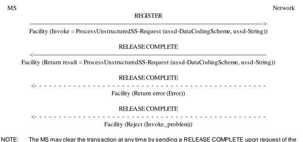
Figure 6.1: Mobile initiated USSD operation, network does not request further information
