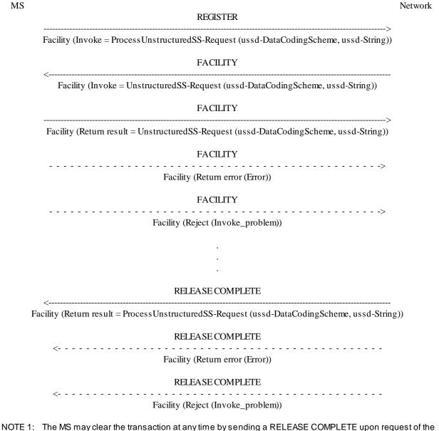
NOTE 1: The MS may clear the transaction at any time by sending a RELEASE COMPLETE upon request of the user.
