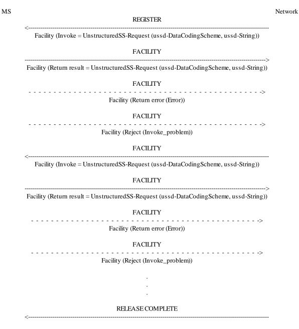
NOTE 1: The MS may clear the transaction at any time by sending a RELEASE COMPLETE upon request of the user.
