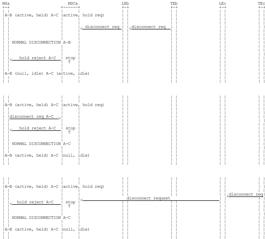
Figure 2.3 (sheet 3 of 3): Information flow for call hold
