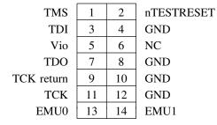
All JTAG signals have 2.8 V native logic levels and are tolerant of 3.3 V, but NOT any higher voltages. The JTAG interface is needed very rarely; it is not needed at all in normal usage and even during intensive firmware development a need for JTAG arises only very rarely.
